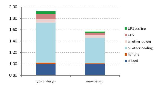
Note that the typical new data center PUE of 1.57 is significantly better than the installed base value of 1.92. In fact, the energy bill for a given IT load is directly proportional to the PUE, so we can say that a current generation data center will typically have an 18% reduction in energy use for the same IT load, when compared with the typical installed base. We can now add a third entry to the chart to show the PUE improvement of using ecomode, as shown in Figure 5.
