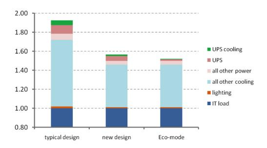
When co-mode is engaged, the UPS loss drops from 5% to 2% (corresponding to an efficiency improvement from 95% to 98%), but the PUE falls only from 1.57 to 1.52. This represents a savings of total energy use of 3.3%. In this analysis, it is assumed that the data center is operating at 50% load using modern UPS systems. The result is that, as a rule:
