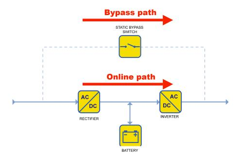
There are two main paths that can supply the load, the online (double conversion) path and the bypass path. Note that the load is connected to the raw<sup>2</sup>, unconditioned mains power when the bypass is active. The following table shows when each path is used in both online and eco-mode operation:
