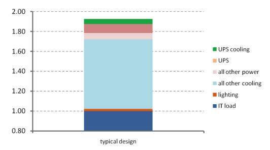
Note that the vertical axis of the graph begins at 0.8 – not at zero – to show detail. The IT load always contributes exactly 1.0 to a PUE value.
