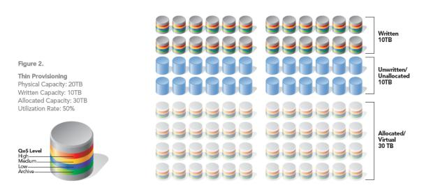
Figure 2. Thin provisioning with Pillar Axiom 600 results in efficient storage utilization.
