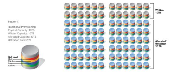
Figure 1. Traditional provisioning results in excess storage capacity.
